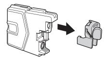
Each colour has its own correct position. Insert the ink cartridge in the direction of the arrow on the label.
